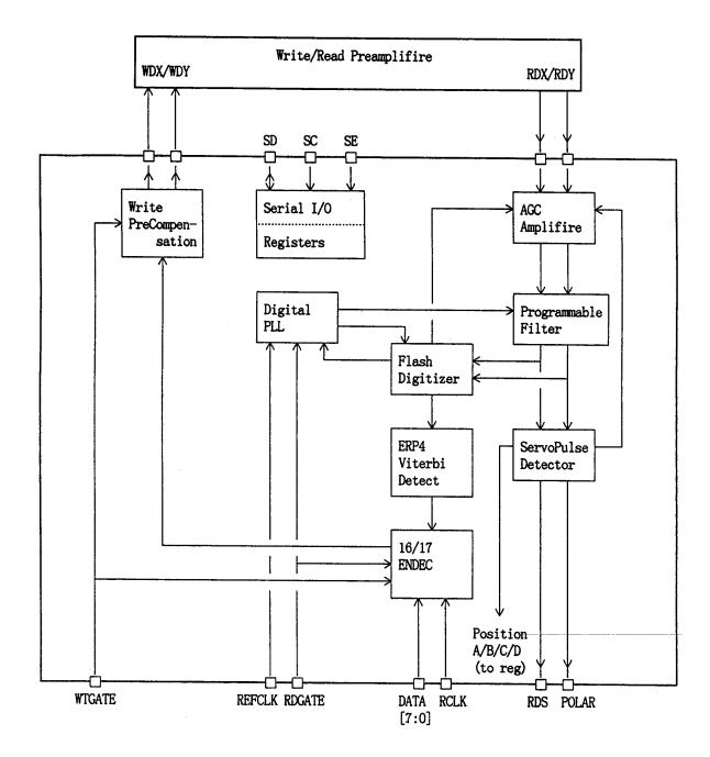
Figure 4.4 Read/write circuit block diagram
